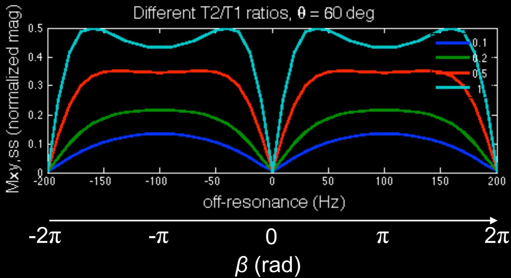
Recall  $\beta = 2\pi \Delta f \times \text{TR}$  and  $\Delta f = \gamma B / 2\pi$
