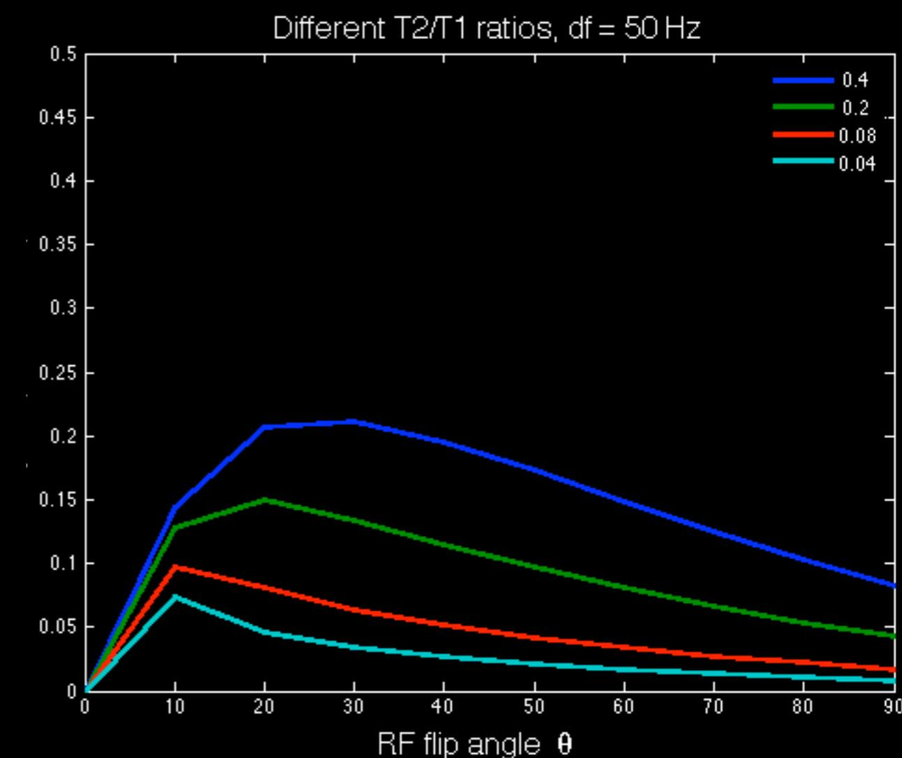
$T_1 = 100, 200, 500, 1000 \text{ ms}$ ,  $T_2 = 40 \text{ ms}$
