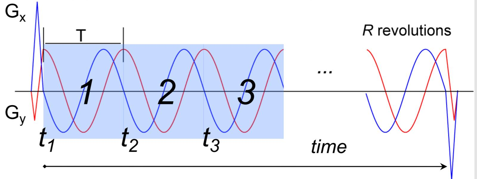
Encodes  $(k_x, k_y, time)$  simultaneously
