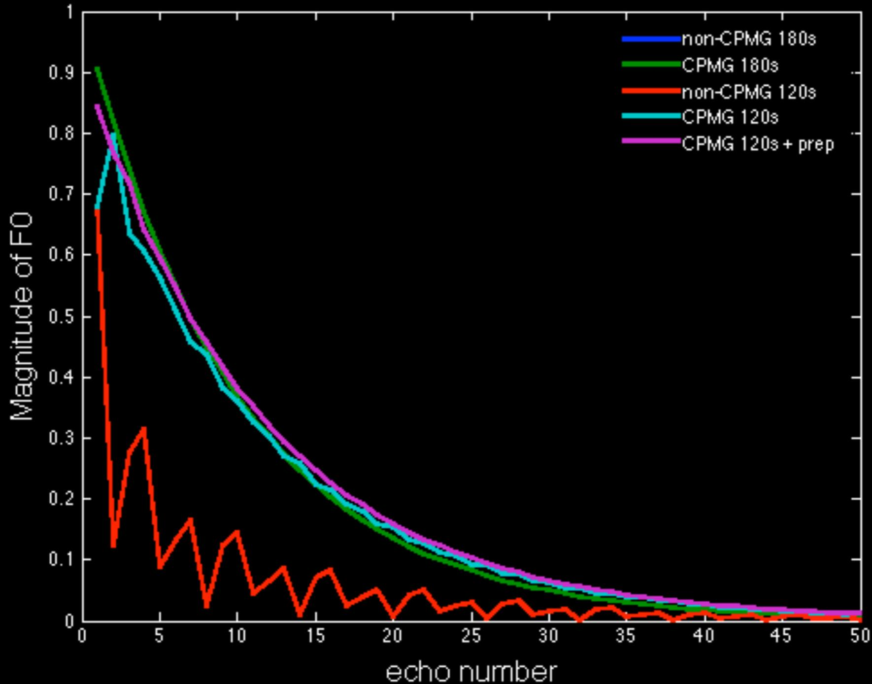
$T_1 = 1000$  ms,  $T_2 = 100$  ms, ETL = 50, ESP = 10 ms
