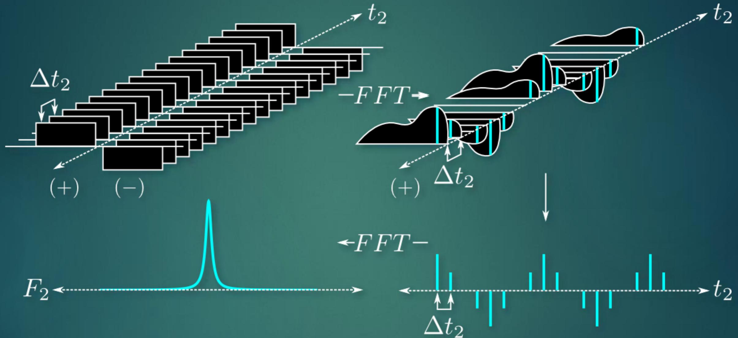
the repeated nature of the readout gradients spatially encodes as a function of time
