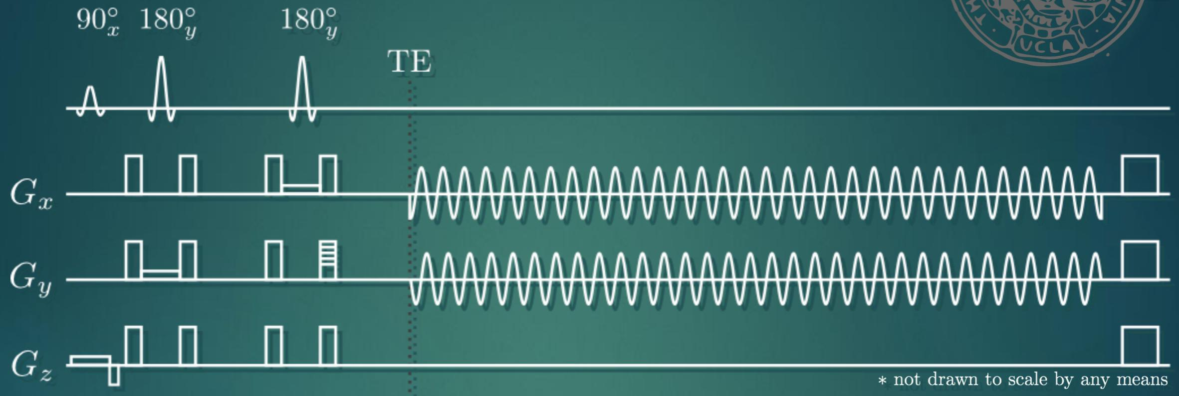
The use of a concentric k-space trajectory is readily applied to ordinary CSI sequences
