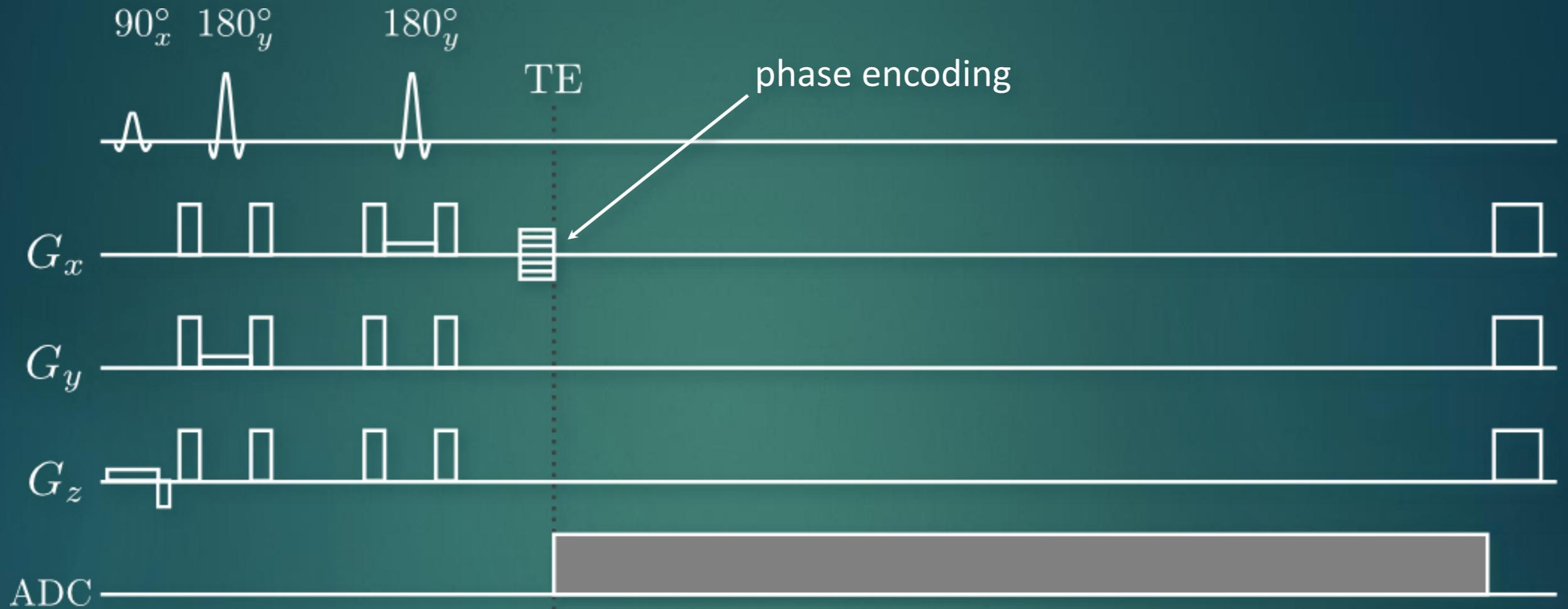
sample 1D spectroscopic imaging pulse sequence
