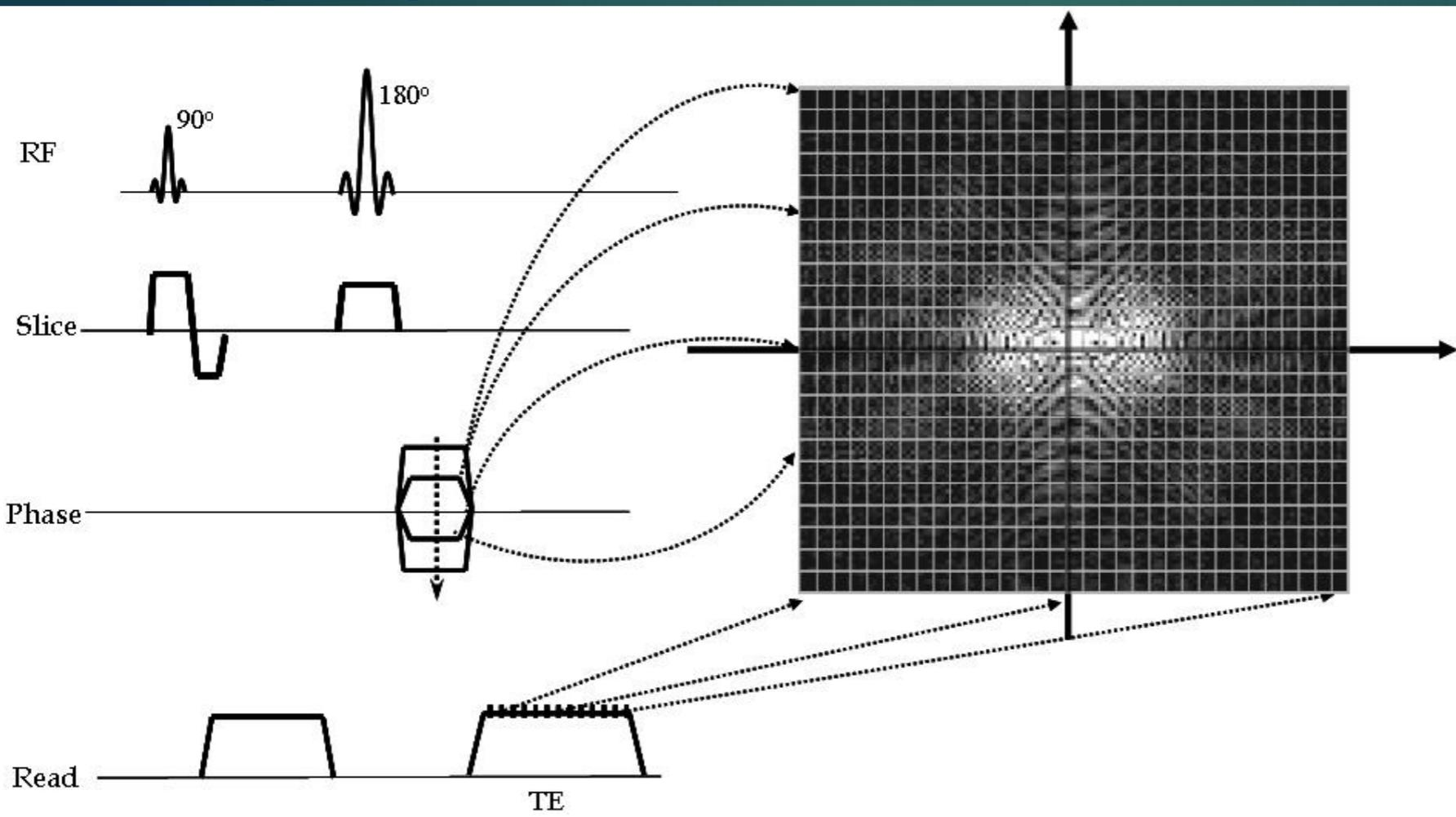
Gradient applied along the y-axis will cause the spins to precess at a frequency determined by their y position, and is called phase encoding. Next a gradient is applied along the x-axis and the spin-echo is collected. The frequency components of the echo gives information of the x-position and the phase values give information of the y-position.
