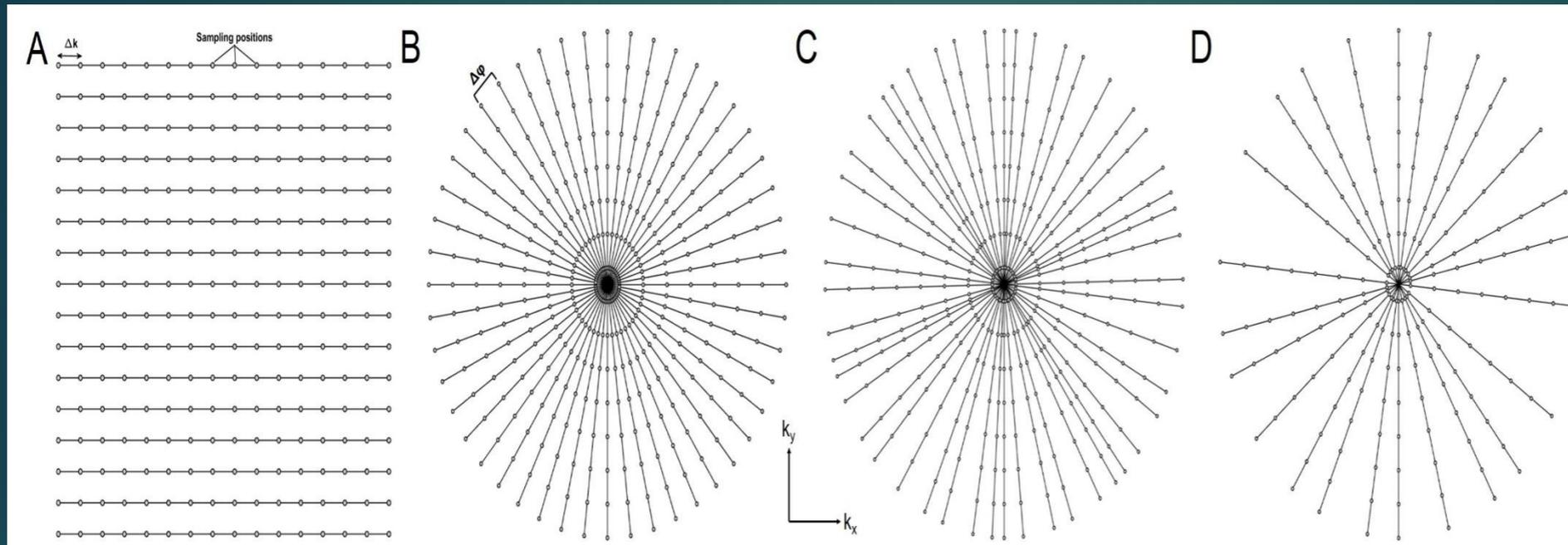
Sampling schemes using **(A)** Cartesian encoding; **(B)** radial encoding; **(C)** Golden angle radial projections successively incremented by  $111.25^\circ$ ,  $\Delta k = \text{FOV}$ . No of spokes,  $n_s = (\pi/2) * n$ , where  $n$  = base resolution, distance between spokes  $< \Delta k$ . **(D)** Undersampled radial acquisition (2X) compared to **(C)**.
