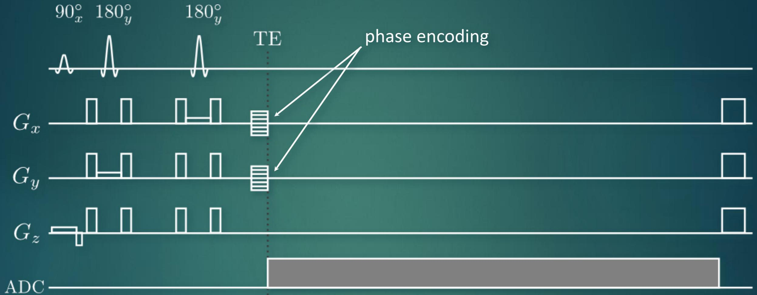
sample 2D spectroscopic imaging pulse sequence
