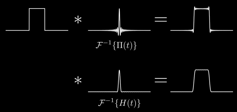
Hamming window can be used to reduce ringing
